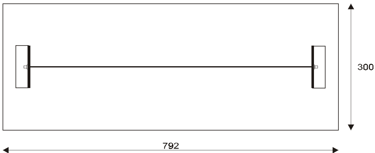
Figure H.4: Top view of the jig (all dimensions in mm)
