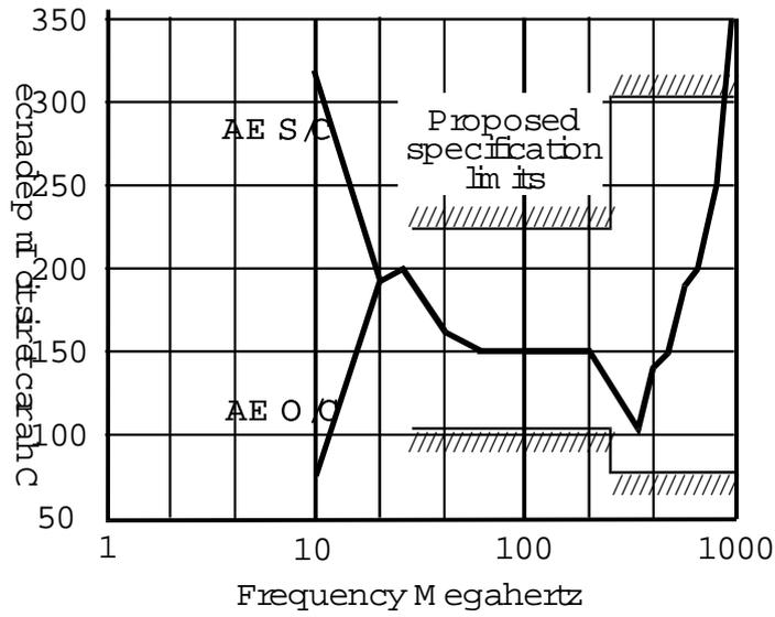
Figure 6 C/M Characteristic Impedance of clamp filter
