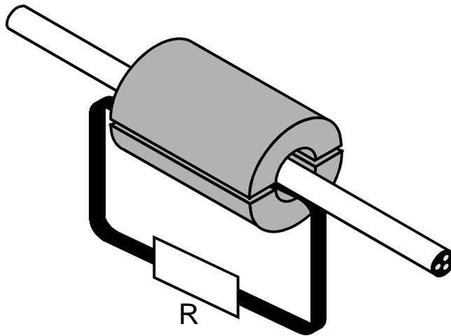
Figure 2 Principle of series-impedance compensation
