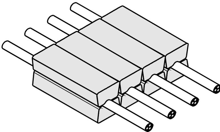
Figure 5 Shunt loading of cables in a duct
