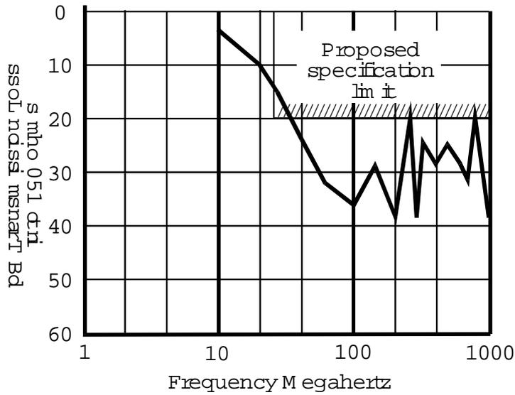
Figure 7 C/M transmission loss of clamp filter
