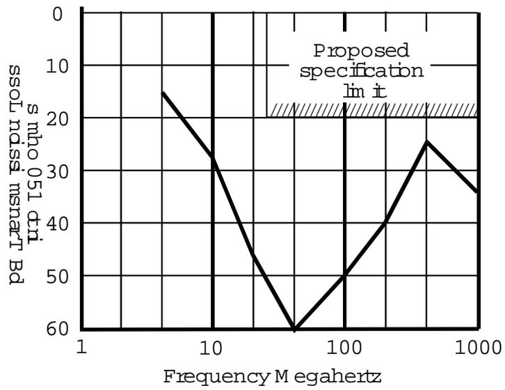
Figure 4 C/M transmission loss of boxed filter
