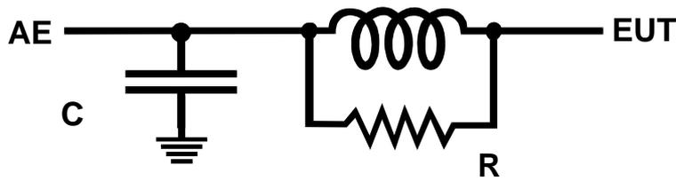
Figure 1. Single section common-mode equivalent circuit
