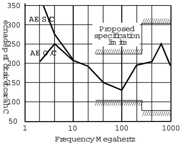
Figure 3 C/M Characteristic Impedance of boxed filter
