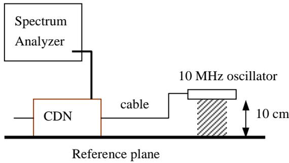
Figure 3. Conducted RF emission test set-up
