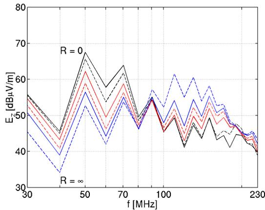
Figure 2. Spectrum of a 10 MHz oscillator measured in a SAR with various CM termination impedances.
