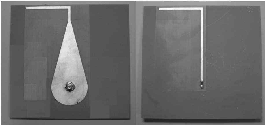
Figure D.5—Front and back sides of planar dipole (dipole ‘B’ in D.4.2 and Figure D.9)
