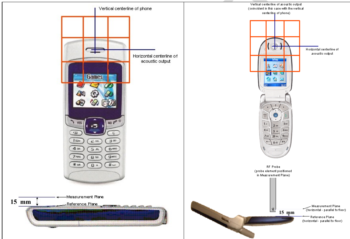
Figure A.2—WD reference and plane for RF emission measurements
