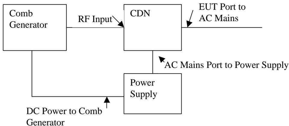
The comb generator, CDN and power supply were all placed on the 80 cm high non-conducting table with the CDN mounted on top of the comb generator chassis. The CDN and comb generator were bonded together with copper tape along two sides. The power supply was placed on top of the table in front of the comb generator / CDN combination. The only cable extending below the surface of the table was the power cord connected between the EUT port of the CDN and the power receptacle on the turntable.
