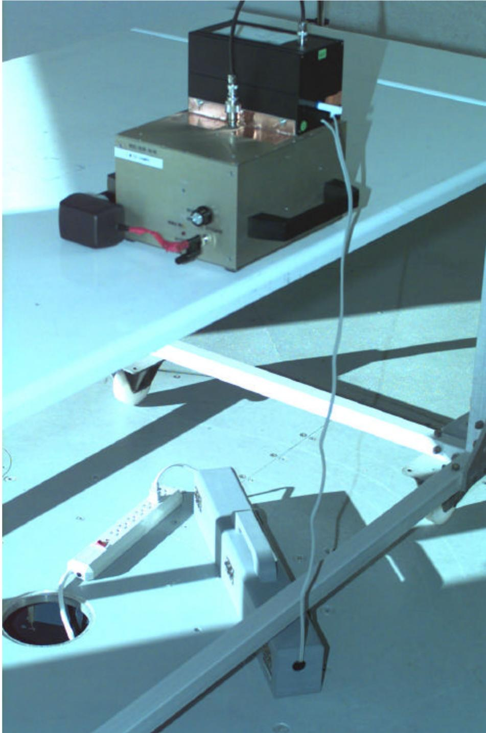
**Photo #2 - Ferrite Clamp on Power Cord**
