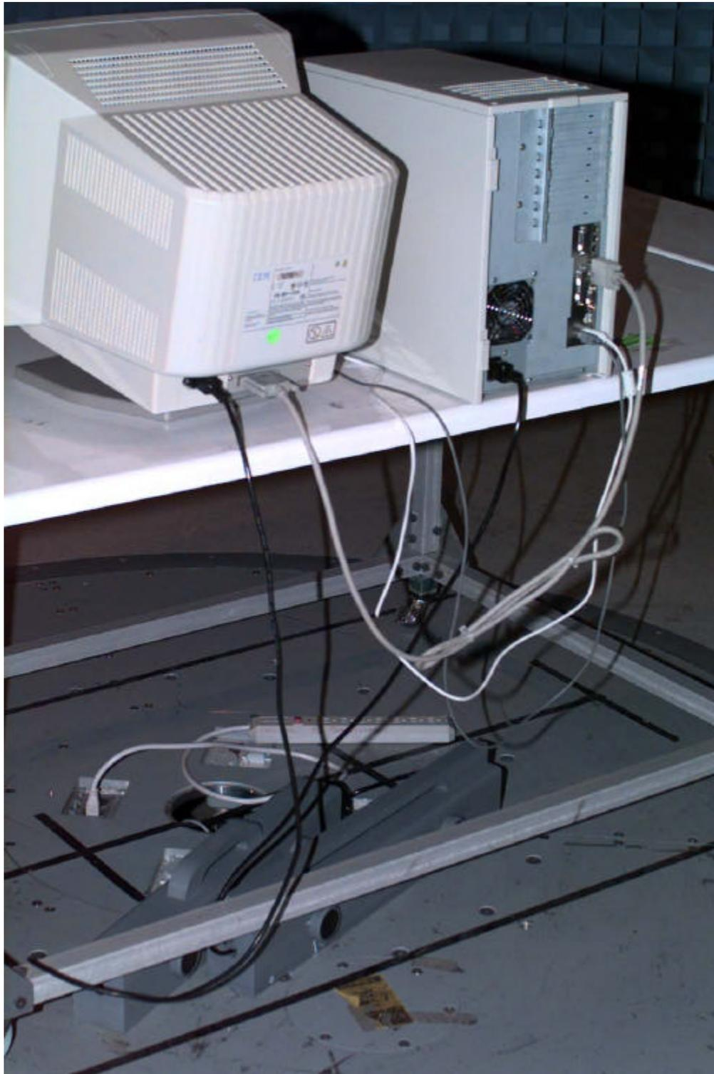
**ATX System w/ Ferrite Clamps on Power Cords**
