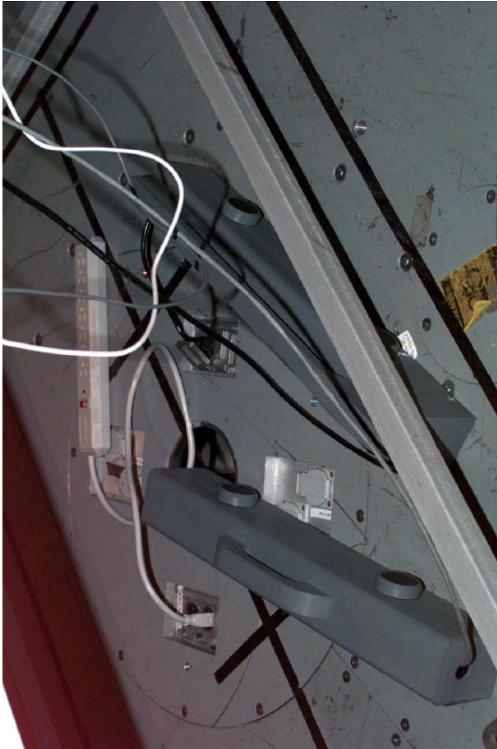
**NLX System Ferrite Clamp Detail**
