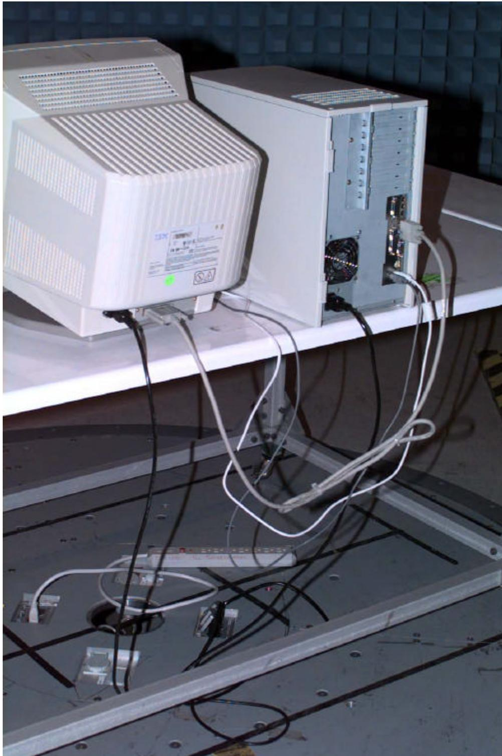
**ATX System w/o Ferrite Clamps**
